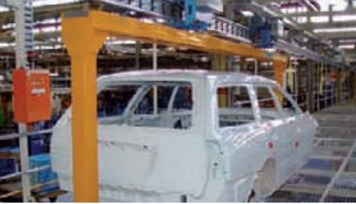
Electrified monorail system with IPT®-Rail and iDAT
