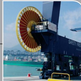
Power cable reel with fiber optics for STS Cranes
